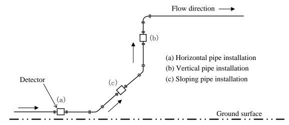
Figure 4.7 Detector Piping Orientation
